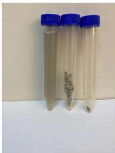
Figure 4: Wastewater, paper fiber residues and stainless steel particles obtained by the deinking process, respectively, from left to right
