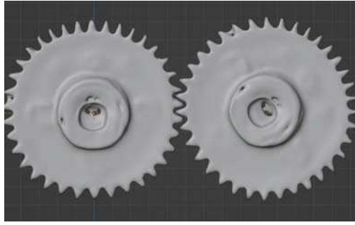
Figure 3: Luma AI model - tooth alignment between two gears
