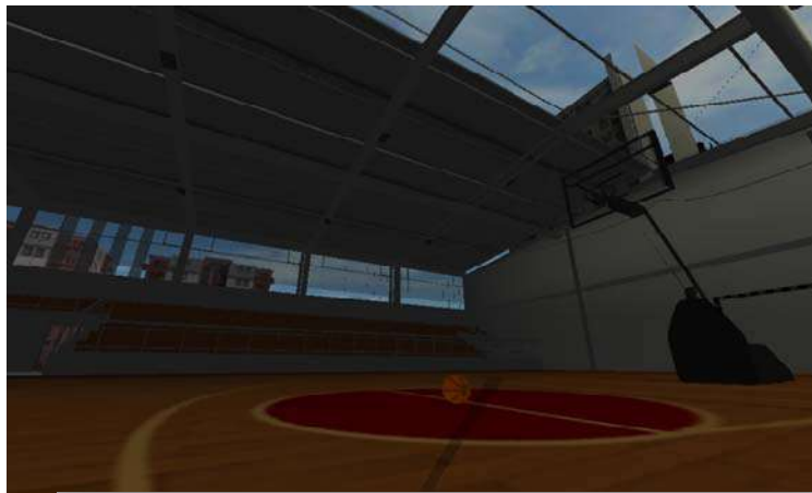
Figure 9: Simulation of the illumination in the interior of the sport hall in daylight, modulated when passing through the electrochromatic film in a shaded state. The film's transmission coefficient main value is 57.06%. The solar range AM 1.5 is fallen light and the interior lighting is switch off
