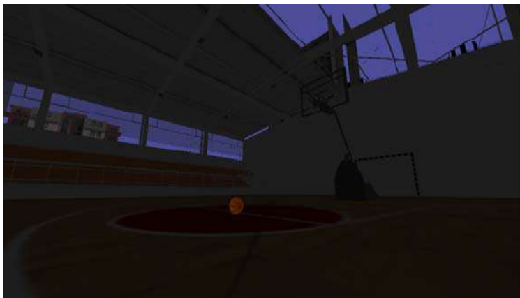
Figure 10: Simulation of the illumination in the interior of the sport hall in daylight, modulated when passing through the electrochromatic film in a coloured state. The film's transmission coefficient main value is 20,0%. The solar range AM 1.5 is fallen light and the interior lighting is switch off
