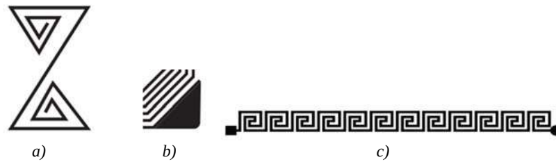
Figure 1: Patterns for printing a) sample for resistance measurement, b) sample for rub test, c) sample for double folding test
